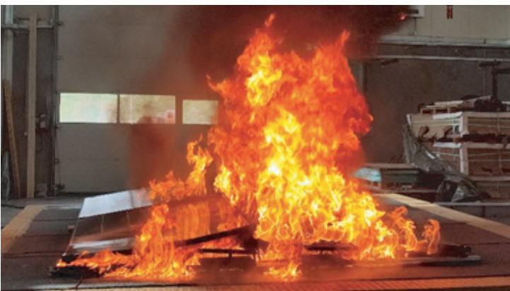
Figure 6 - E-W format test without ArcBox showing rapid development of fire across the roof covering behind the panels
