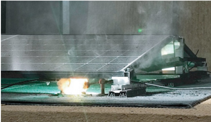
Figure 4 - E-W format test without ArcBox and high energy arc visible
