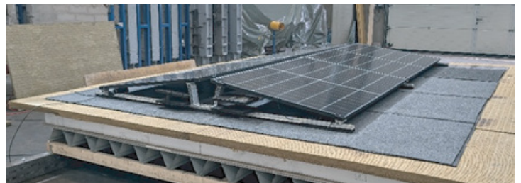
Figure 3: Flat roof solar configurations. East-West facing configuration
